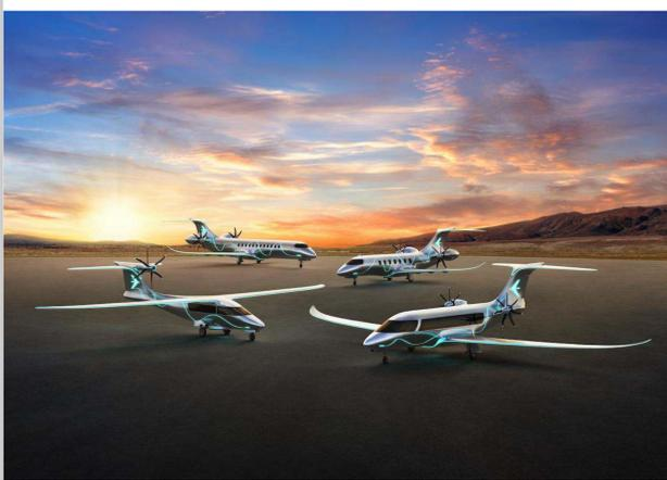
Energia concepts [clockwise from front right]: hybrid-electric E9-HE, all-electric E9-FE, hydrogen-turbine E50-H2GT and hydrogen-electric H19-H2FC.
